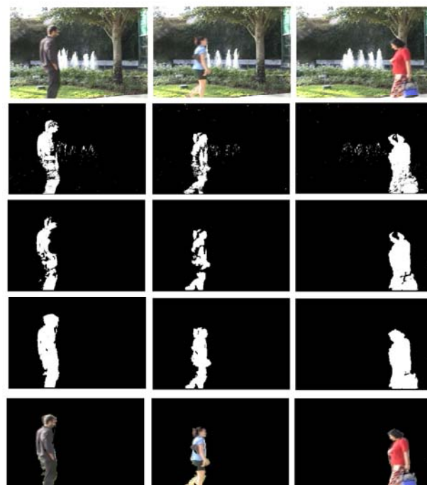
Fig.3 The top row shows the original images of the fountain sequence, the second row shows the results obtained using a five-component Gaussian mixture model, and the third row shows the results obtained using Sheikh's algorithm. The fourth row shows the results obtained by the proposed method, and the fifth row shows the original masked image
