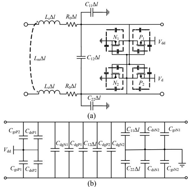
Fig.4 (a) Lumped equivalent circuit of loaded transmission line with length  $\Delta l$ ; (b) Equivalent capacitance circuit
