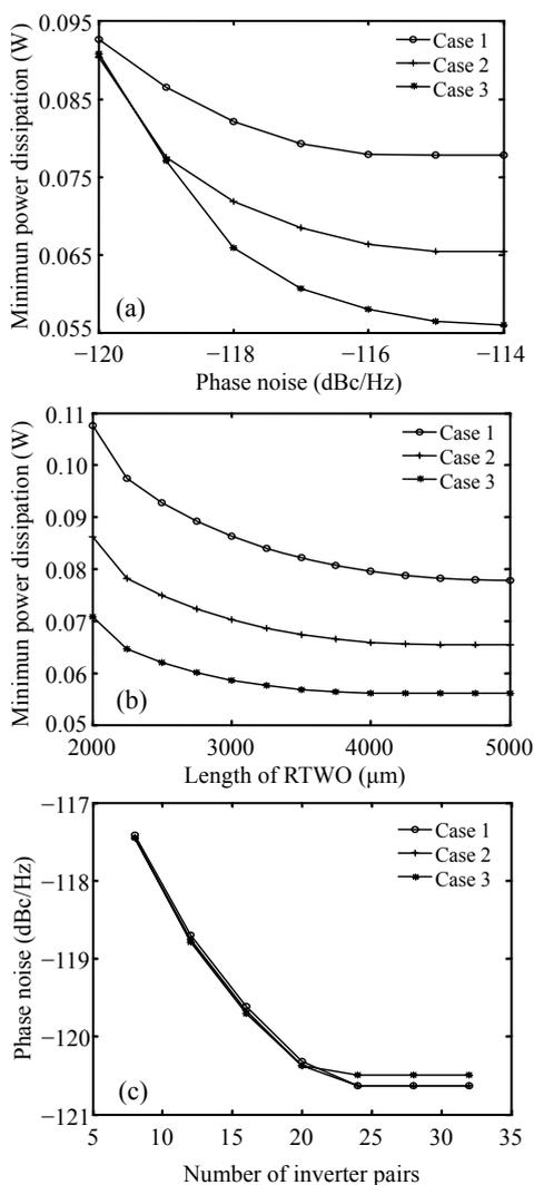
**Fig.7 Trade-off curves of (a) power dissipation vs. phase noise, (b) power dissipation vs. length of RTWO, and (c) phase noise vs. the number of inverter pairs**
