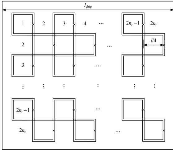
Fig.2 Structure of the rotary traveling wave oscillator array (RTWOA)
