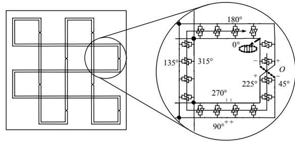
**Fig.1** Circuit diagram of the rotary traveling wave oscillator array (RTWOA)
