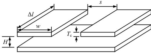
Fig.3 Structure of differential transmission lines
