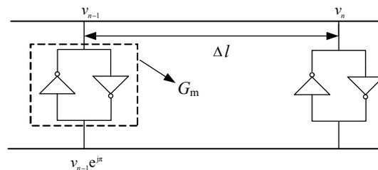
Fig.5 A short section of the transmission line
