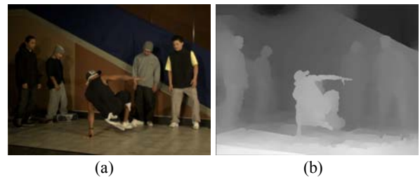
Fig.1 The first image with depth from camera 4 of a test sequence ‘breakdancers’
