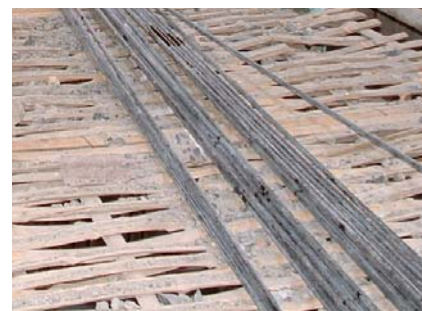
Fig.4 10-mm diameter CFRP bar
