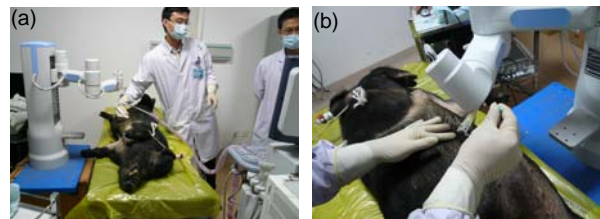
Fig. 10 Experiment on animals (pig). (a) Ultrasound scanning; (b) Robot assisting needle placement
