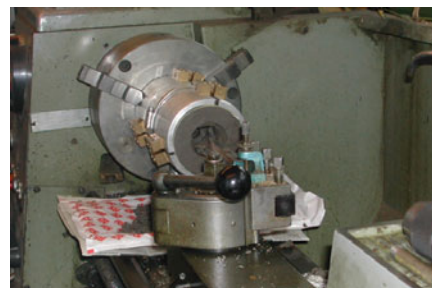
Fig. 17 Intact mudrock sample preparation for hollow cylinder apparatus (HCA) testing Internal hollow cylindrical cavities are bored out employing lathe and drill sizes are expanded (Ann-Minh, 2006)
