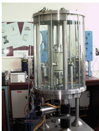
Fig. 16 Photograph of Imperial College Mark II HCA used to test London clay samples (OD=100 mm, ID=60 mm, h=200 mm) (Nishimura et al. , 2007)
