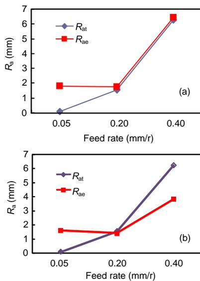
**Fig. 4** Surface roughness deviation using (a) insert TPMR 160308 (insert 60°) and (b) insert CNMG 120408 (insert 80°)
