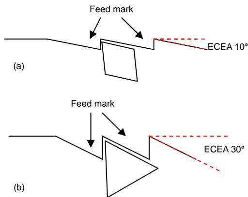
**Fig. 6** Feed mark formations of (a) CNMG 120408 (rhombus) and (b) TPMR 160308 (triangle)
