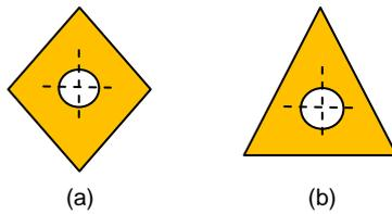
Fig. 2 Insert shapes of (a) ‘C’ type and (b) ‘T’ type
