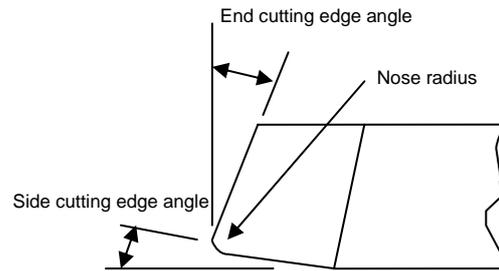
Fig. 1 End cutting edge angle (ECEA)
