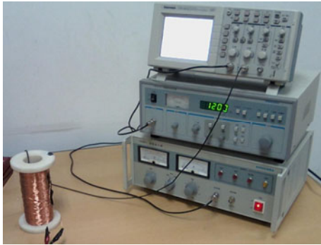
Fig. 3 Experimental setup for determining the relationship between V_{ME} (mV) and B (mT)
