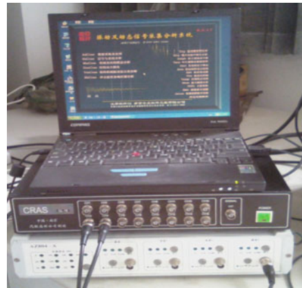
Fig. 7 Signal conditioning and data acquisition instruments
