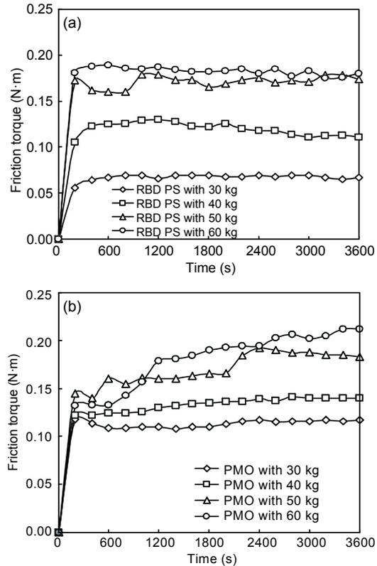
Fig. 2 Friction torque distribution vs. time for various normal load conditions for RBD PS (a) and PMO (b)
