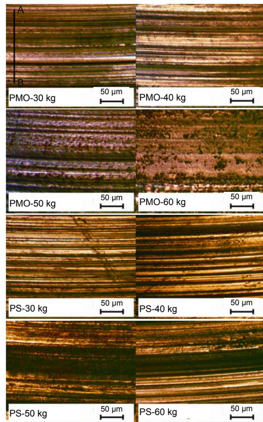
Fig. 6 CCD micrographs of the wear scar on the ball specimen
