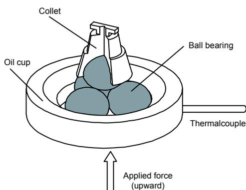
Fig. 1 Schematic sketch of a four-ball tribotester
