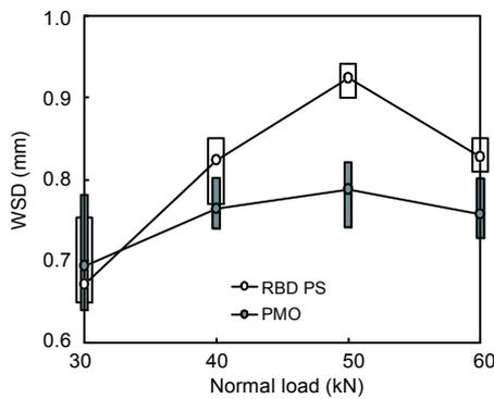
Fig. 4 Wear scar diameter (WSD) distribution
