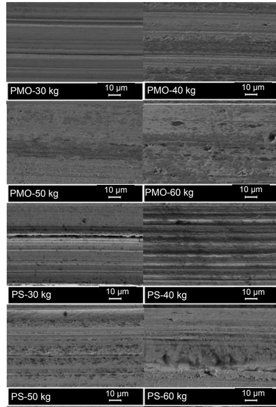
Fig. 7 SEM morphologies of the worn surface
