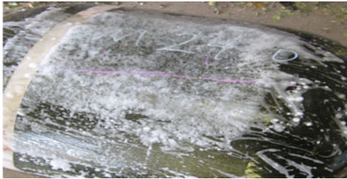
Fig. 10 Failure after fatigue test
