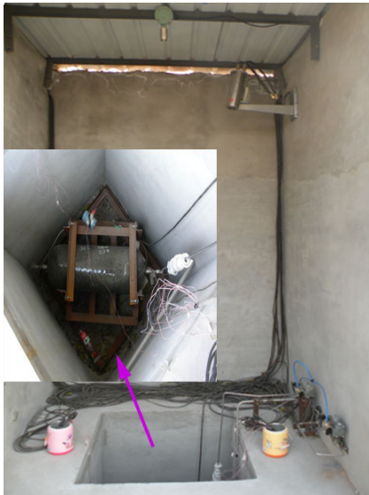
Fig. 7 Fatigue test of composite hydrogen storage vessel
