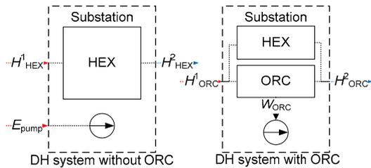
Fig. 4 Heat transfer and power consumption in two DH systems with and without ORC
