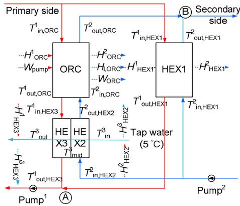
Fig. 9 DH system with HEXs and ORC in parallel connection (scenario 4)
