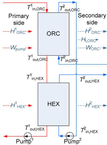
Fig. 8 DH system with HEX and ORC in series connection (scenario 2)
