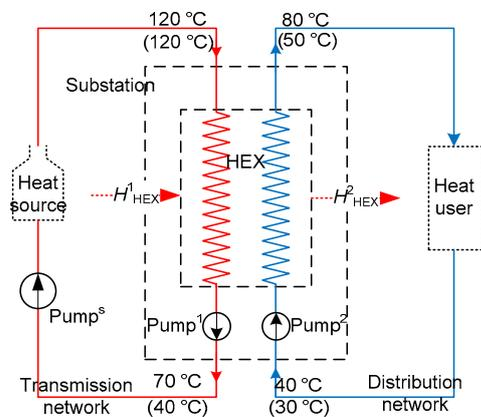
**Fig. 2** A traditional substation in DH
