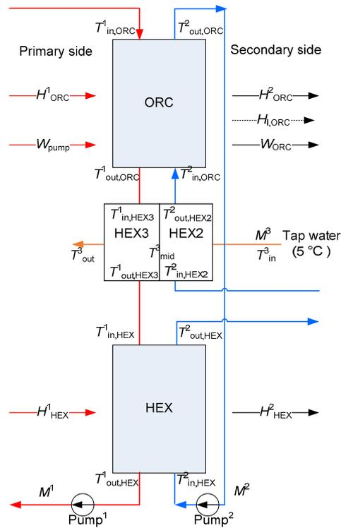
**Fig. 10 An improved configuration for a LTDH integrated with an ORC in series**
