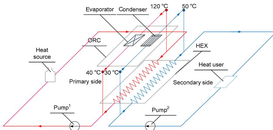
Fig. 3 A LTDH system integrated with ORC
