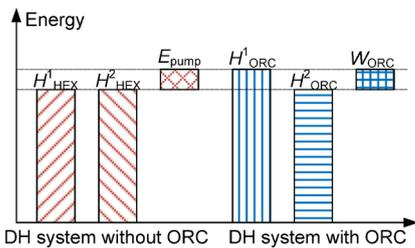
Fig. 5 Energy balance of two DH systems with and without ORC
