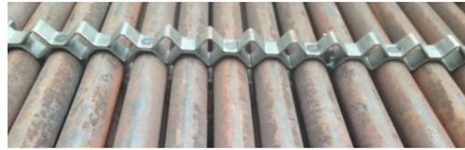
**Fig. 1** Picture of tube bundle supported by the HCB
