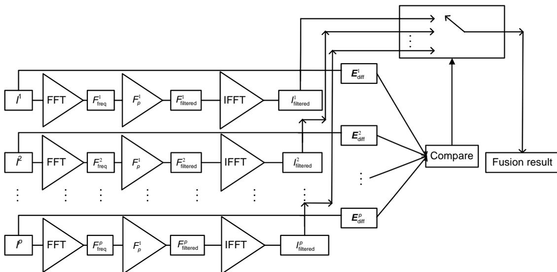
Fig. 1 Schematic diagram of filtering in frequency domain and synthesis in space domain (FFDSSD)
