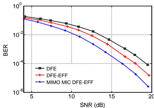
**Fig. 5 BER performance of the proposed MIMO MIC DFE-EFF compared with conventional DFE, and DFE-EFF over MIMO frequency selective Rayleigh channel**
