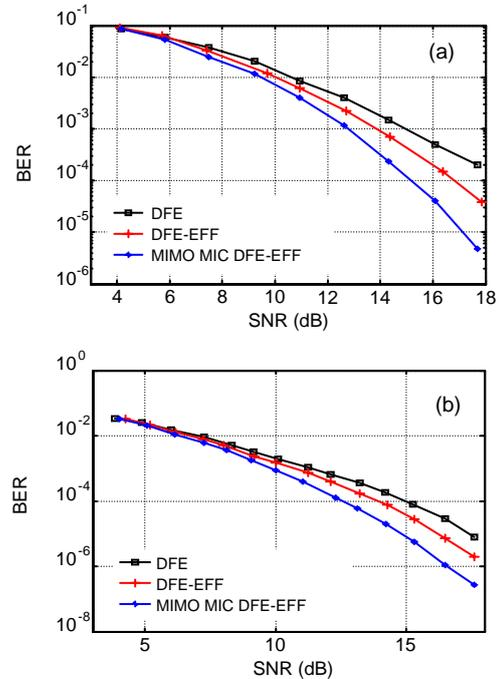
**Fig. 6 BER performance of our proposed MIMO MIC DFE-EFF compared with conventional DFE and DFE-EFF over MIMO frequency selective Rayleigh channel, for four (a) and eight (b) spread factors**
