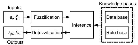
Fig. 3 Structure of the fuzzy proportional and derivative (PD) self-tuning regulator
