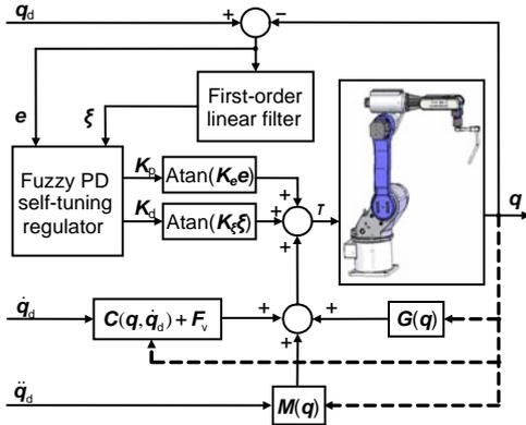
Fig. 2 Block diagram of the proposed output feedback tracking (OFT) controller
