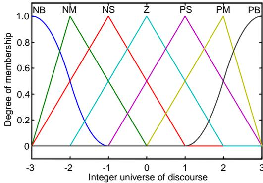
Fig. 4 Membership functions for  $e_i$ ,  $\zeta_i$ ,  $k_{pi}$ , and  $k_{di}$
