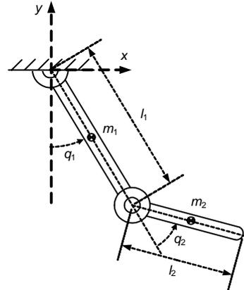
Fig. 5 A two-link direct-driven robot manipulator
