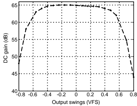
Fig. 15 First operational transconductance amplifier (OTA) voltage gain versus different output swings
