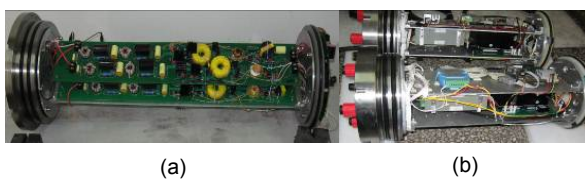
Fig. 6 Prototypes of the medium voltage power converter (a) and two control systems (b)
