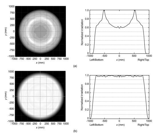
Fig. 10 Illuminance distribution of the target plane: (a) before optimization; (b) after optimization
