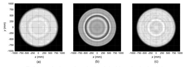
Fig. 5 A comparison between the equal angle method and the equal arc-length method (a) The irradiance map generated by the lens model constructed directly from profile data points in software Rhinoceros; (b) The irradiance map generated by the equal angle method; (c) The irradiance map generated by the equal arc-length method
