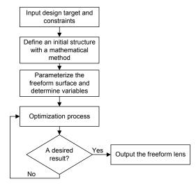
Fig. 1 Flow chart of the design method
