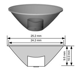
Fig. 9 Model of the freeform lens
