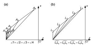
Fig. 4 Methods of optimization points selection: (a) equal angle method; (b) equal arc-length method
