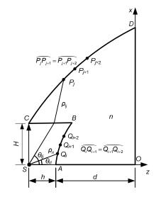
Fig. 7 Optimized variables selection of freeform lens
