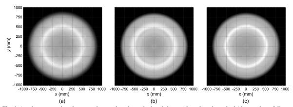
Fig. 6 Another comparison between the equal angle method and the equal arc-length method (the number of discrete optimization points on the lens' profile is 11, and other parameters are the same as in Fig. 5)
